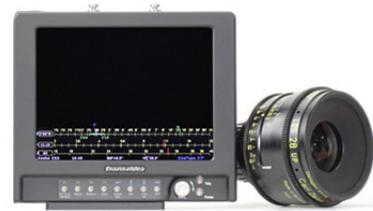
The CineHD display scales on the screen reproducing the Focus, Iris, and Zoom engravings. Two operating modes: Mobile where the focus/iris/zoom scales are moving as on a physical lens; Static where the cursors are moving on the fixed scales.
